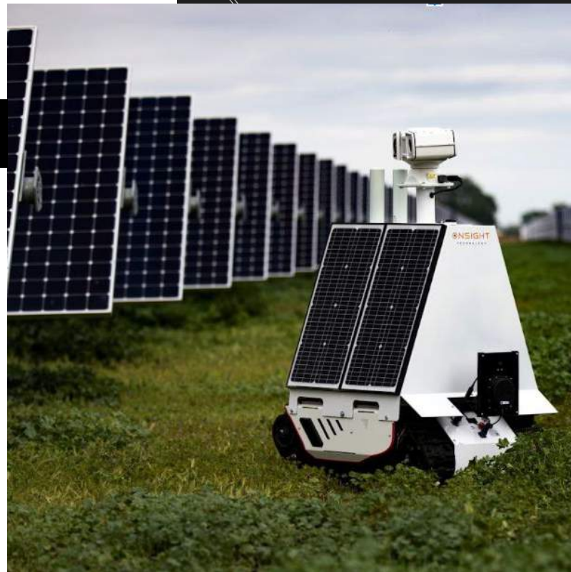
Onsite Technology uses DroneDeploy with their ground robotics to automate commercial solar inspections.
